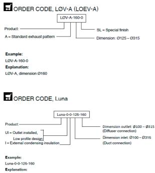
Luna plenum box with duct connection dim. Ø125 and diffuser connection dim. Ø160.
