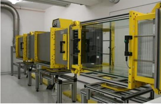
A test rig for testing coarse and fine dust filters according to EN779 is the fundamental component of our filter laboratory.
