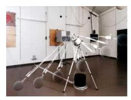
TROX acoustics has 2 reverberation chambers. They meet the recommendations for reverberation chambers in accordance with ISO 3741 (Determination of sound power levels of noise sources using sound pressure - Precision methods for reverberation rooms). In the acoustics laboratory, sound measurements are taken. These measurements are indicative or supportive in the development of new products.
