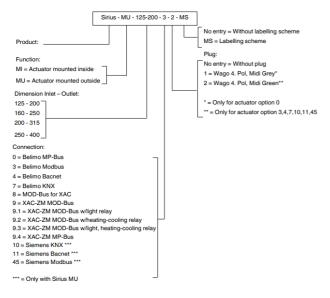
Example: Sirius-MU-125-200-3-2-MS Explanation: Sirius with Ø125 inlet and Ø200 outlet, with Belimo Modbus, Wago-plug mounted, with labeling scheme
