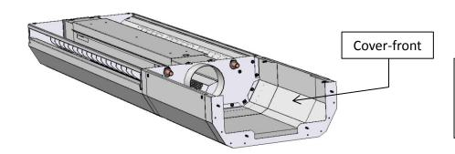
Place the cover-front on the outside of the extension piece and the end piece. Attach the cover-front using screws.
