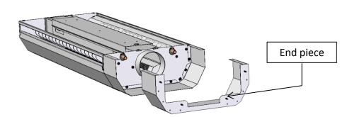
Attach the end piece to the wall in line with the Svalbard F using screws.
