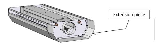
Attach the extension piece to the gable end of Svalbard-F using screws.
