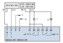
1 Control lamp CLOSED, to be provided by others 2 Control lamp OPEN, to be provided by others Y: 0(2) - 10 V DC Operating range (setpoint) U: 2 - 10 V DC Position feedback (actual value)
