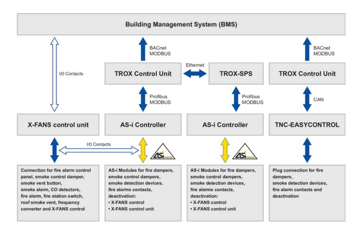
Control and communication modules for smoke control dampers
