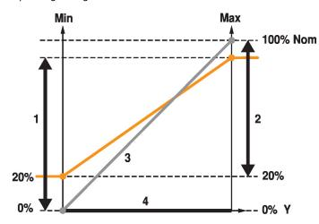
Nominal value (OEM setting) Nom Adjustment range Min 1 Adjustment range Max 2 Feedback U 0...100% Nom 3 Control Y Min...Max 4
