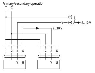
• Max. 8 actuators in parallel • Parallel operation is permitted only on non-connected axes • Do not fail to observe performance data with parallel operation
