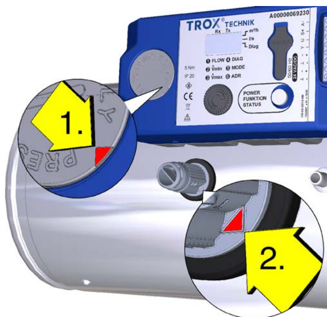
Fig. 30: Plug the control component onto the basic unit
