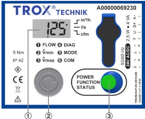
Fig. 23: Display and control elements of the XM0 / XS0 control component
