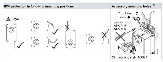
$oldsymbol{\Lambda}$  Not to be used for fixation of the actuator, use anti-rotation-bracket instead.
